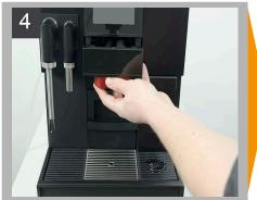
Thoroughly clean SteamJet outlet and cover with the supplied cleaning brush.
